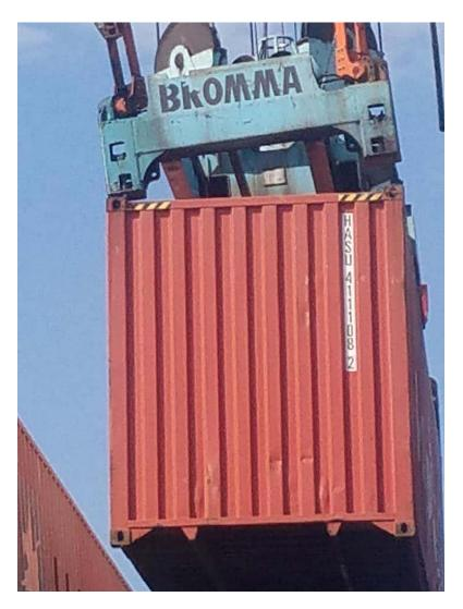
When engaging containers with any spreader device, check your equipment's console lights and get an indication about twist lock engagement. Then, just to be sure, take a test lift and float the load. When lifting containers, being locked into three corners isn't enough. Containers are designed to be top lifted vertically; from all four corners.
