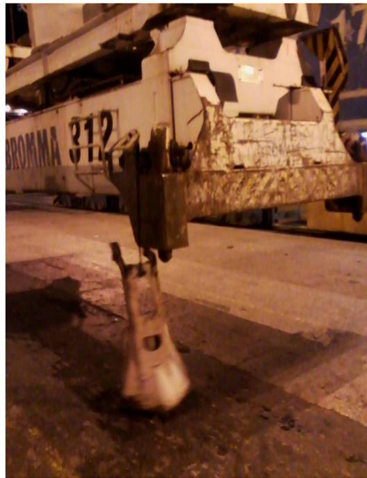
Conscientious condition and maintenance checks should typically provide enough insulation to effectively guard against the obviously dangerous container spreader flipper “free-fall”, an example of which is shown in the photograph *above left*.
