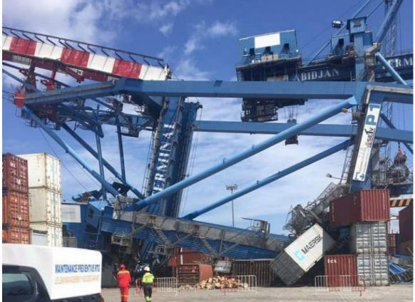
Heavy lift ship **DA ZHI** on May 18 while maneuvering to berth contacted container terminal gantry crane at Berth 21, in **Abidjan, Ivory Coast**. Crane collapsed onto pier area, damages cost said to be sufficient. No information on ship's damages. On a photo collapsed gantry crane.
