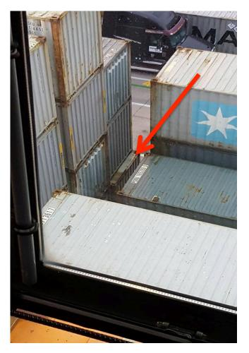
Intermodal containers are designed and constructed to conform to the specifications set out within global (international) standards. They're known as ISO standards. Those ISO standards build a great deal of strength into a container's floor and corner posts, but not nearly as much strength into its sides, ends or top (roof).
