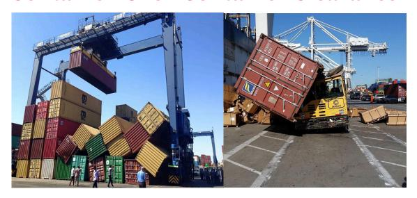
Globally, The ILA~USMX Joint Safety Committee has observed an increased incidence of stowed/stacked containers that are knocked out of position (toppled) by another container being trolleyed along the bridge of ship to shore or yard gantry cranes (RTGs).
