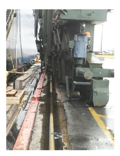
From those sources, we understand that the boom collapsed and folded onto the vessel. We also understand that the resultant forces transmitted down the crane's structure acted in a manner that caused several of the crane's trucks to come off their respective rails (see photo above). Finally, and fortunately, we understand that no workers were injured as a result of this incident.
